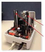
2. This image shows the camera covers off. Two arrows mark where the cameras are located. You will notice a piece of glass with a white strip behind it.
